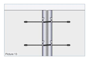
False positions in vertical direction up to 30 mm are covered by a design value.
