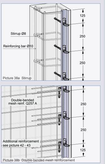
Alternatively the stirrups can be replaced by a comparable mesh reinforcement (Picture 37b and 38b).
