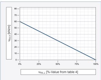
Picture 31 Interaction diagram of the shear forces parallel and right-angled to the joint
