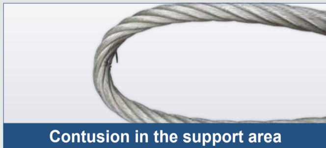
Loosening of external layer
