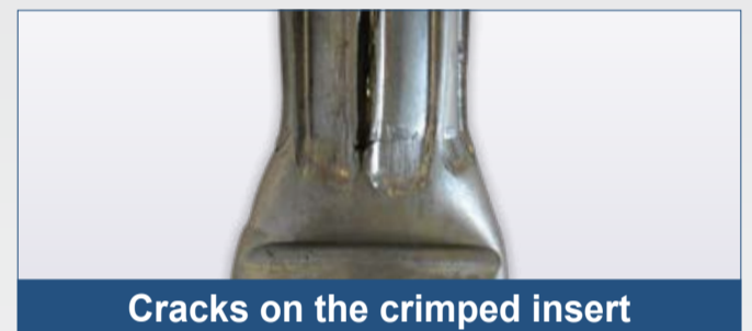
Pull-out of wire rope from crimped part
