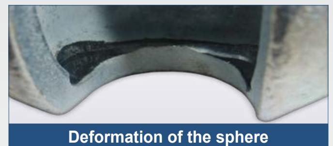
Crack in sphere
