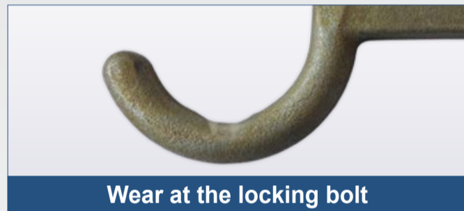
Deformed coupling link
