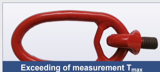
Deformed chain link
