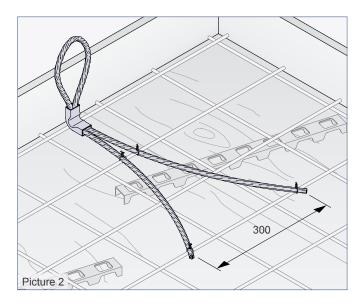
If a significant corrosion occurs to the protruding parts of the Angled loops a transport of the elements is not allowed anymore.
