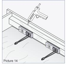
As the bonding effect of lightweight concrete is different to normal concrete, we recommend the use of our special Connecting loop version (e.g. 54VSM120LB) for lightweight aggregate concrete with open structure (LAC).
