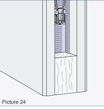
Like the Connecting loops also the Connecting rails can be produced as a special version for lightweight concrete (e.g. 84VS201005LB). In this case, to the reference number "LB" must be added.
