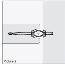
Pay attention to the fact that Connecting loops must not be fixed directly to the formwork without using a timber board, then no grouting channel is created (page 11).
