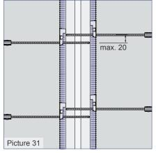
The plastic cover of the installed rail must be released at one rail end. Then, it can be removed easily from the rail. The loops are now folded right-angled to the (metal) box or rail.
